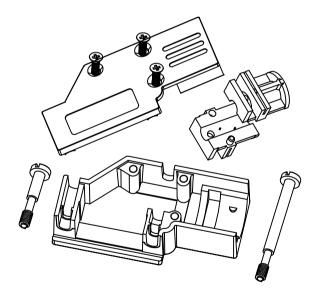
BACKSHELL: MATERIAL: PLATING: 4-40 THUMBSCREWS: HOUSING SCREWS: COMPRESSION INSERT: OPERATING TEMP: DIE CAST ZINC ALLOY NICKEL PLATED STEEL-Zn PLATED STEEL-Zn PLATED ABS,UL RECOGNIZED -40°C TO+120°C
